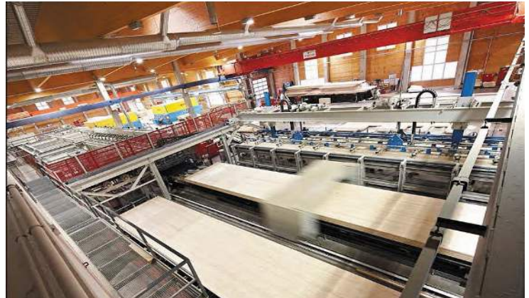
CLT production with automated equipment and precise pre fabrication
